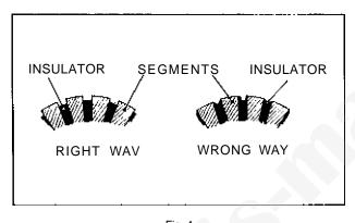
Fig. 4 Method of undercutting commutator insulation
