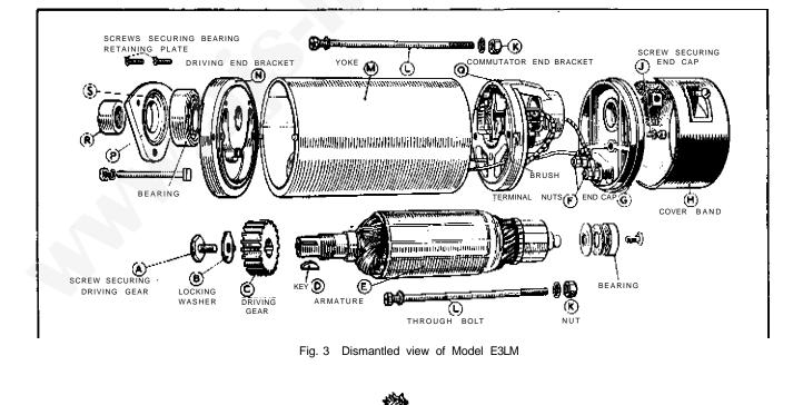
(viii) Take out the screw securing the green field coil lead with the yellow sleeve to commutator end bracket and remove the end bracket 'Q' withdrawing the connectors through the slot in the Insulating plate.
