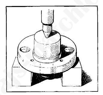
Fig. 9 Replacing the ball race
