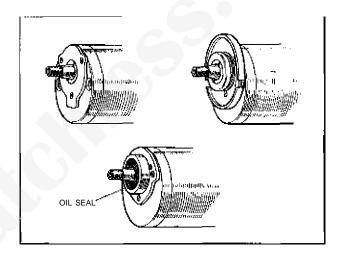
Fig. 1 Various drive-end bearing retaining places
