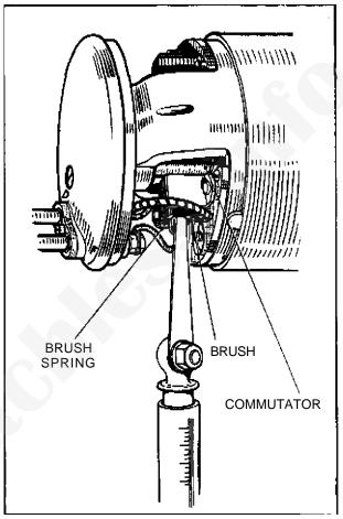
Fig. 2 Testing brush spring tension
