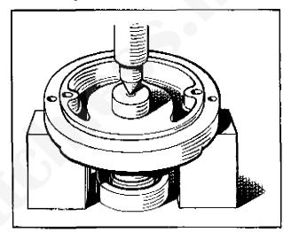
Fig. 8 Removing the ball race
